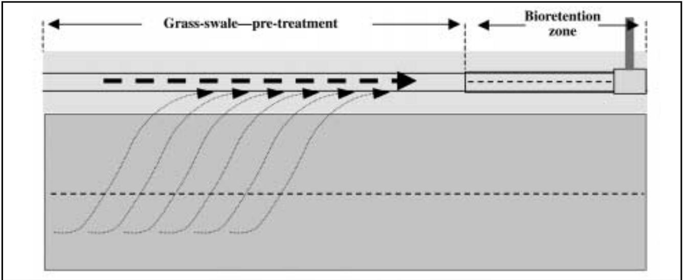
Figure 6.10 Plan illustration of swale drain and bioretention system for managing road runoff
