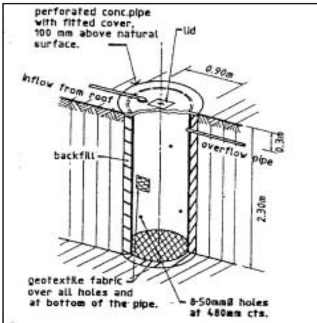
Figure 5.6 Illustration of a perforated retention/overflow well (Argue, 1994)
