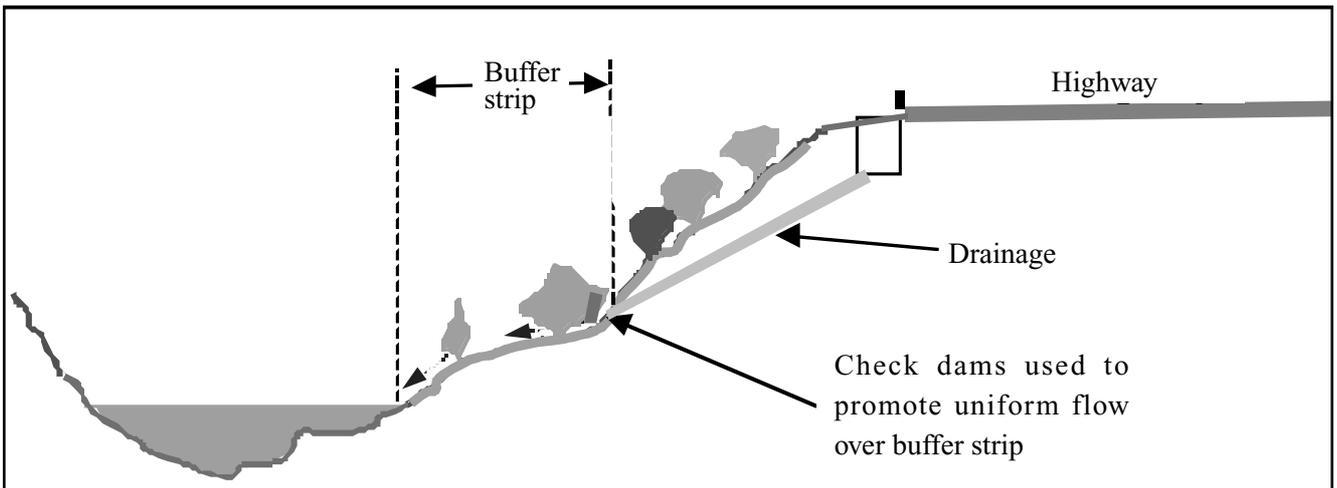
Figure 6.7 Section illustration of kerb and channel & buffer strip runoff management option
