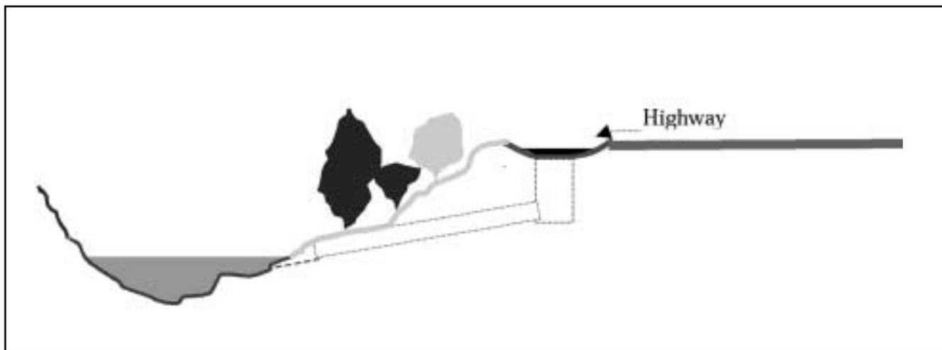
Figure 6.9 Section illustration of swale drain runoff management option
