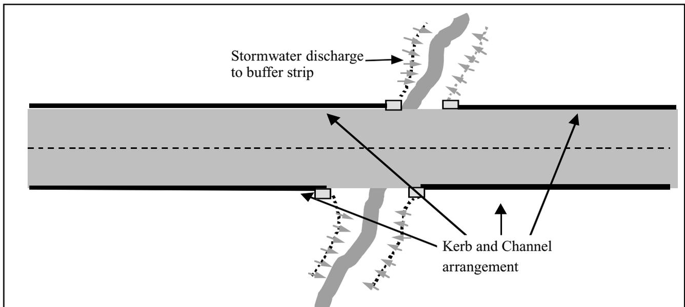
Figure 6.17 Plan illustration of kerb and channel and buffer strip along creek
