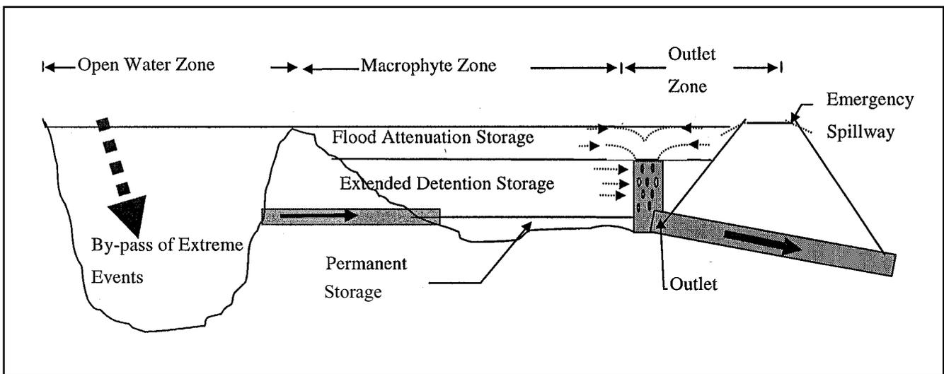
Figure 6.20 Functional zones in constructed wetlands (not to scale)
