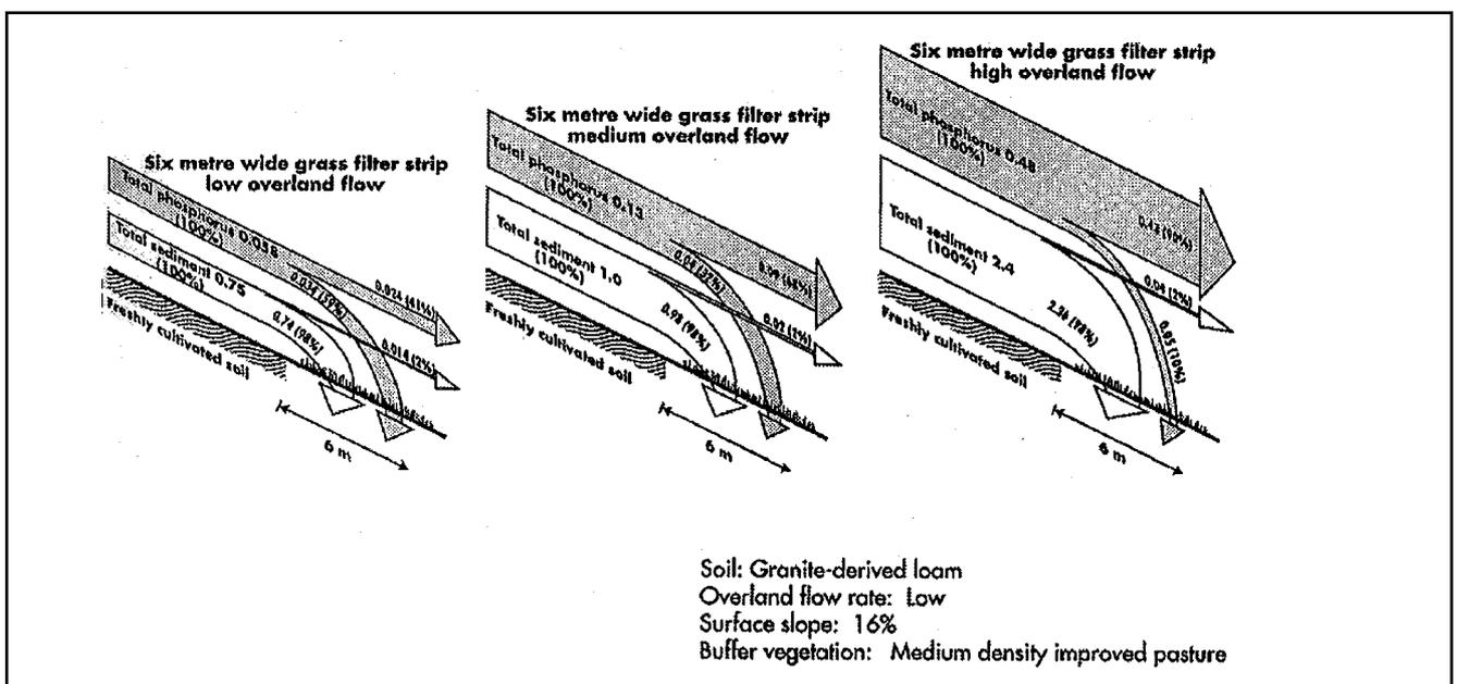
Figure 5.4. Buffer strip effectiveness for sediment and phosphorus removal under a range of sediment input loads and flow conditions (Bren et al., 1997)
