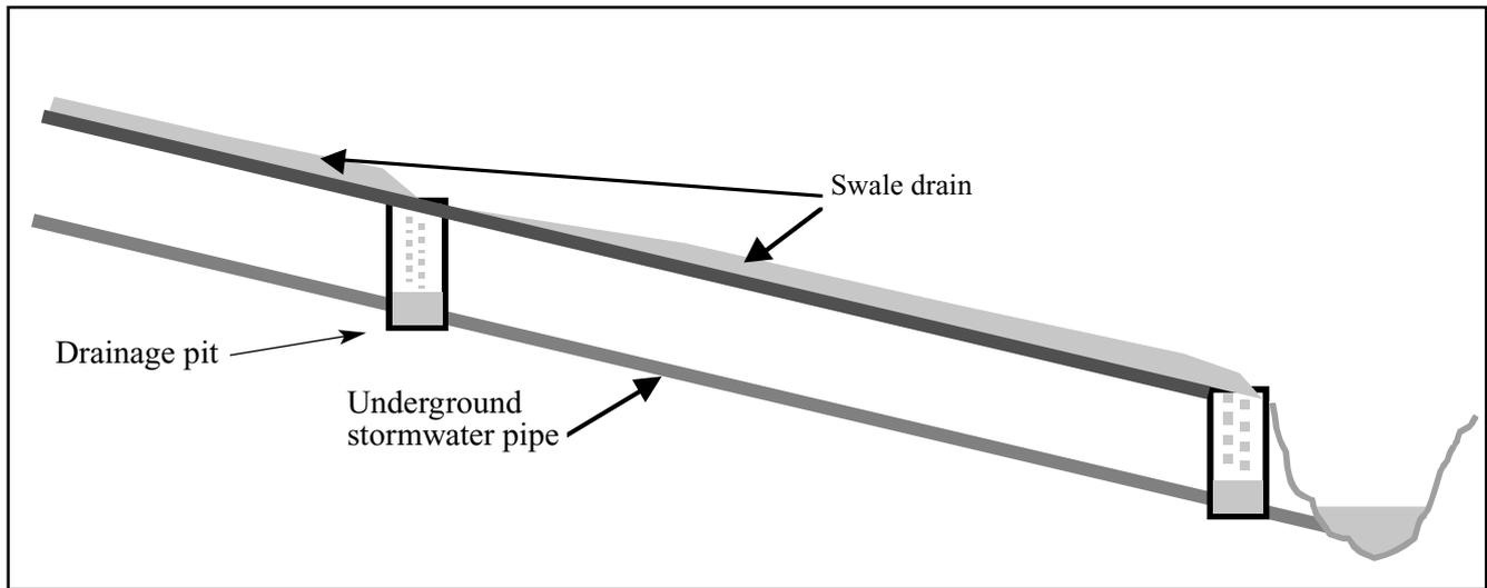
Figure 6.16 Longitudinal illustration of swale drain/underground stormwater pipe system
