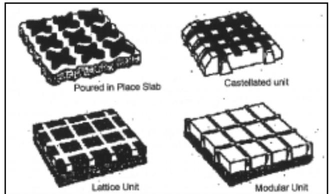
Figure 5.2 Porous pavements are commonly used in car parks and driveways to allow infiltration of rainfall (Schueler, 1995)
