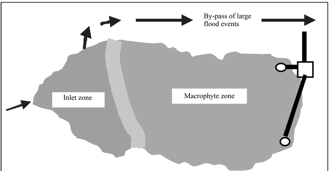
Figure 6.19 Typical layout of a constructed stormwater wetland
