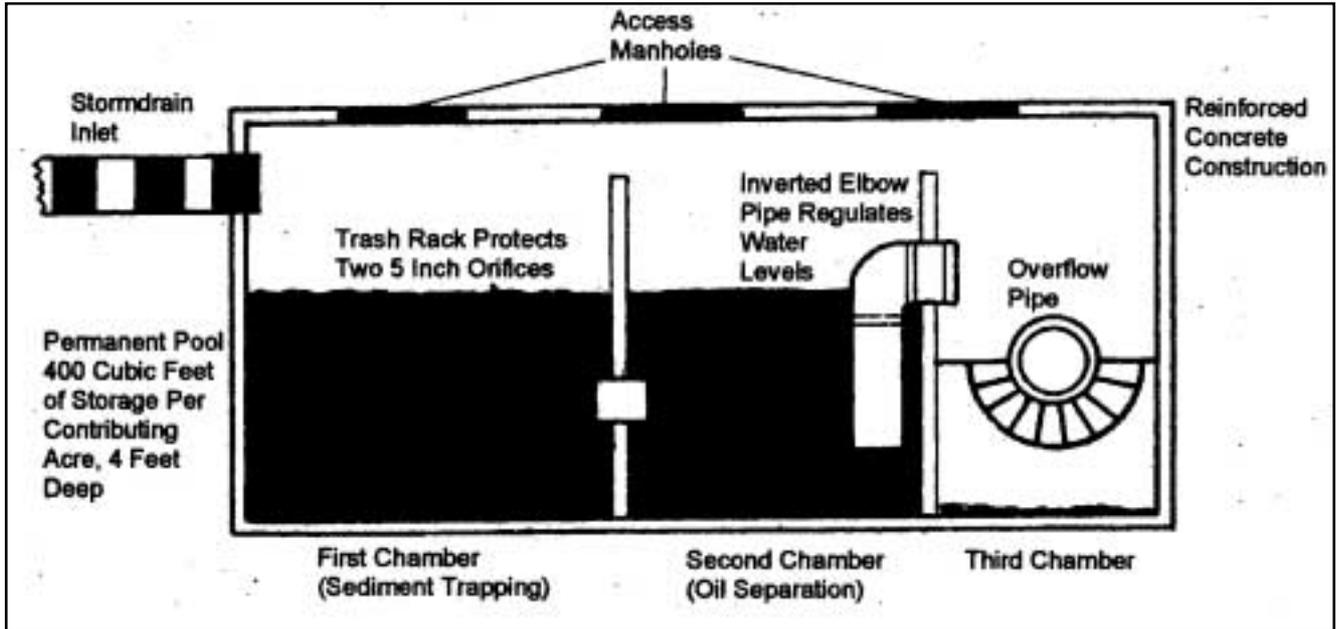
Figure 5.9 Component of an oil and grease trap
