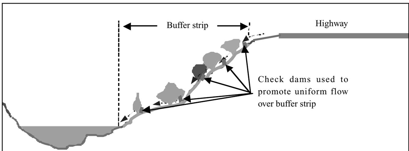
Figure 6.5 Section illustration of buffer strip runoff management option
