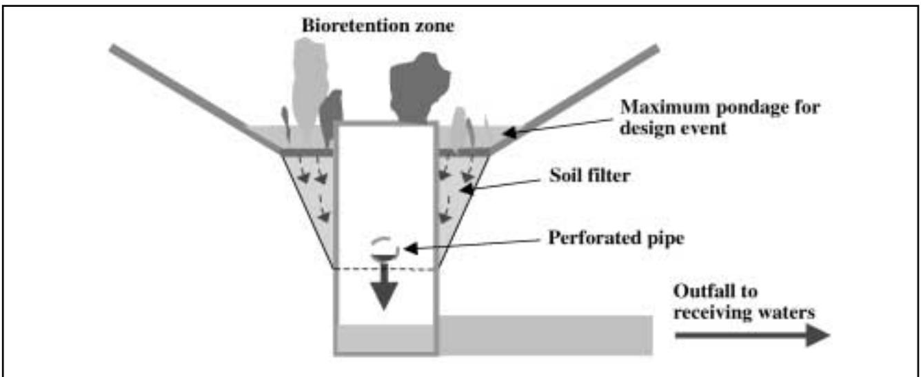
Figure 6.12 Cross section illustration of bioretention media
