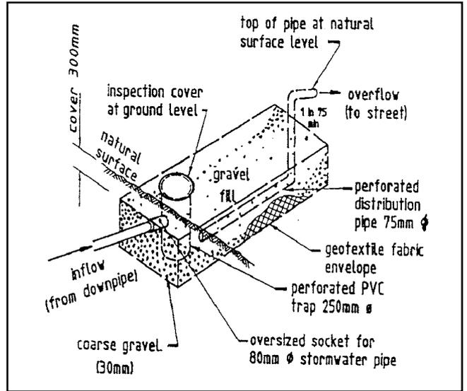
Figure 5.7 Illustration of a shallow retention/overflow trench (Argue, 1994)
