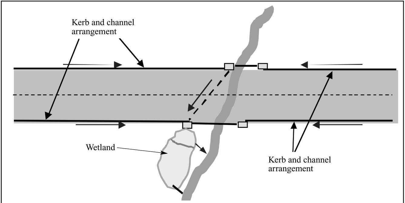
Figure 6.18 Plan illustration of kerb and channel, and constructed wetlands
