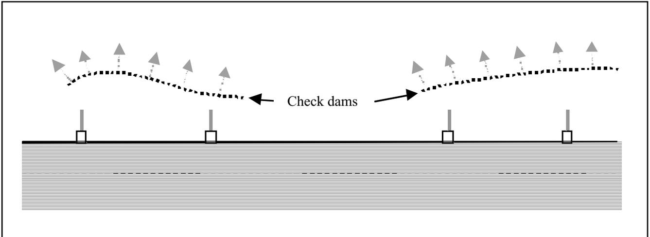
Figure 6.6 Plan illustration of kerb and channel & buffer strip runoff management option
