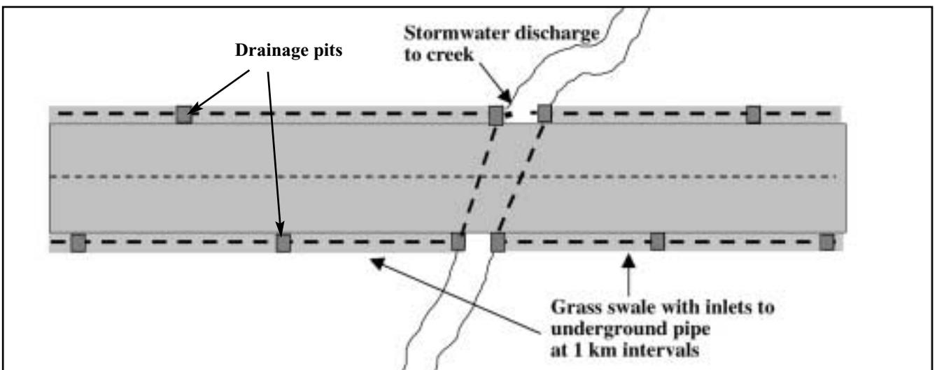
Figure 6.15 Plan illustration of swale drain/drainage pit option
