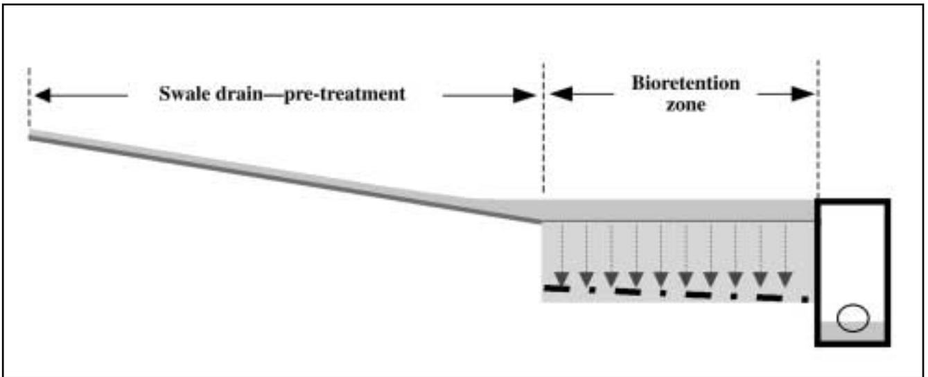
Figure 6.11 Section illustration of swale drain runoff management option
