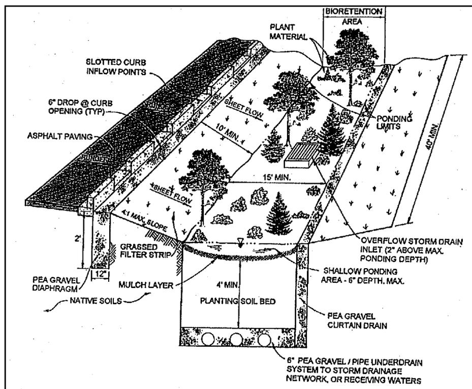
Figure 5.5 Infiltration system used at parking lots with pre-treatment provided by a grass buffer strip (Schueler, 1995)
