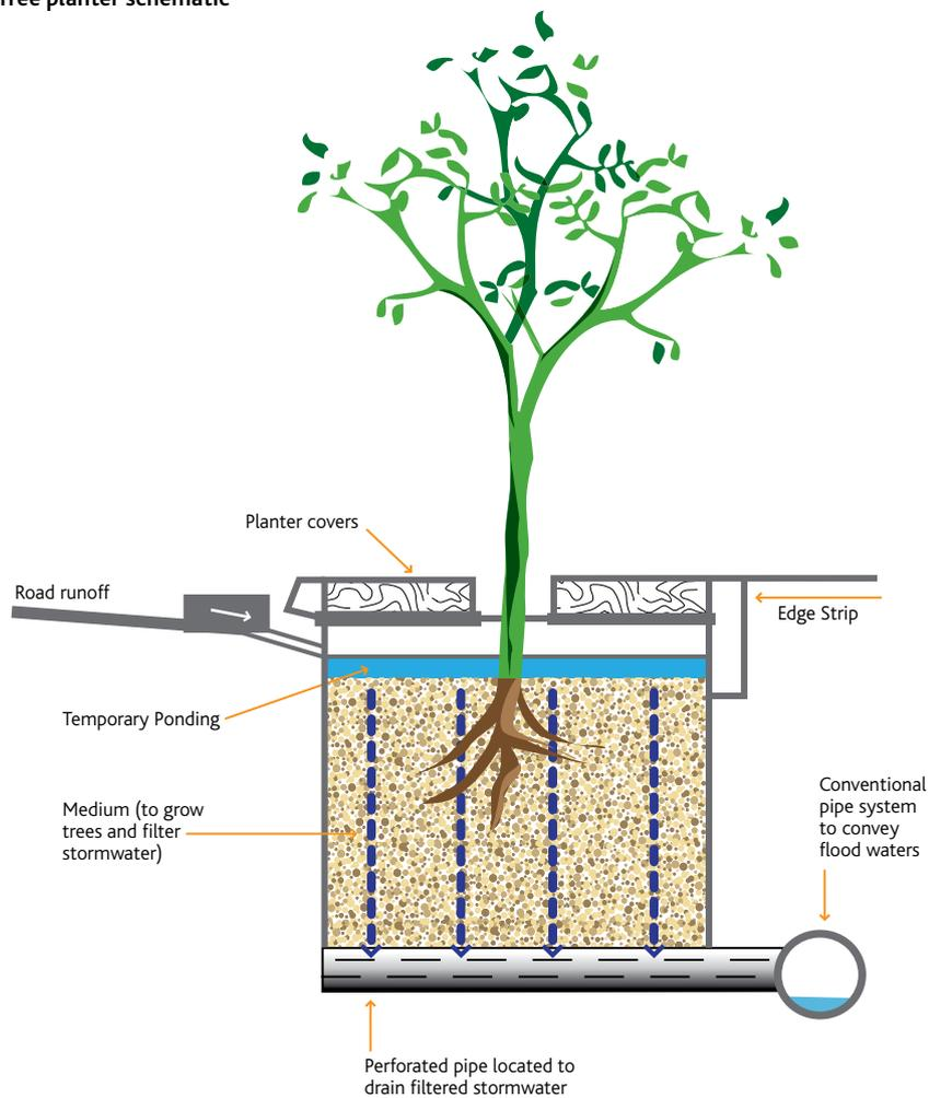
Bioretention tree pits can be installed when street trees are planted. This means that trees are watered by the road runoff which is then filtered through sand before it's released into the stormwater systems. Figure 27 shows a series of street trees – bioretention & conventional.
