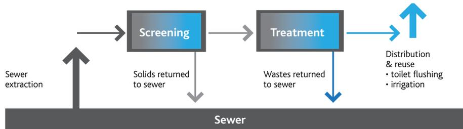
Figure 13 shows a typical water mining treatment systems, consisting of:
