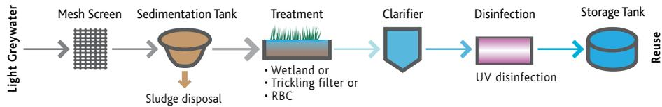
**Mesh screen:** The mesh screen physically traps and removes larger objects from the greywater reuse process.
