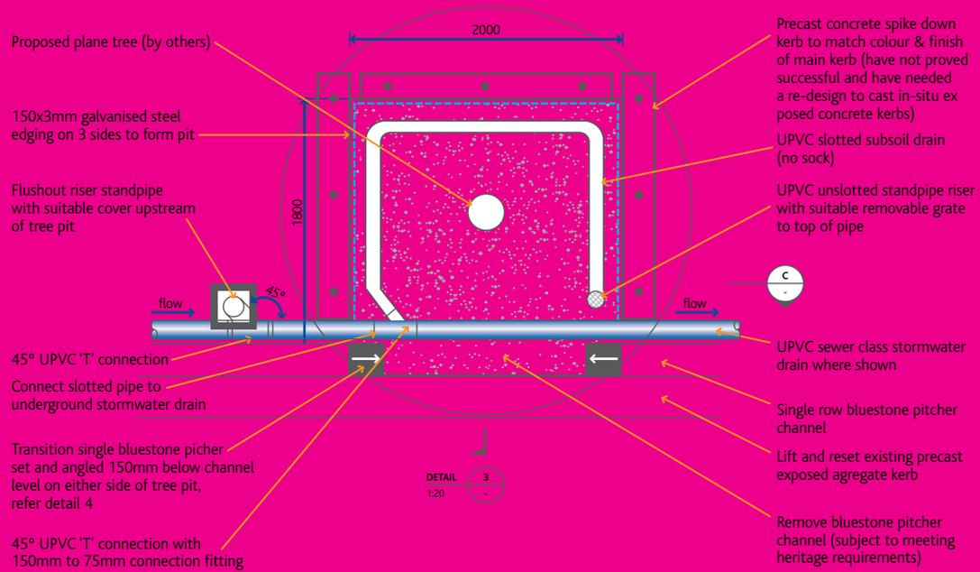
Figure 4: Plan view of raingarden showing surface details
