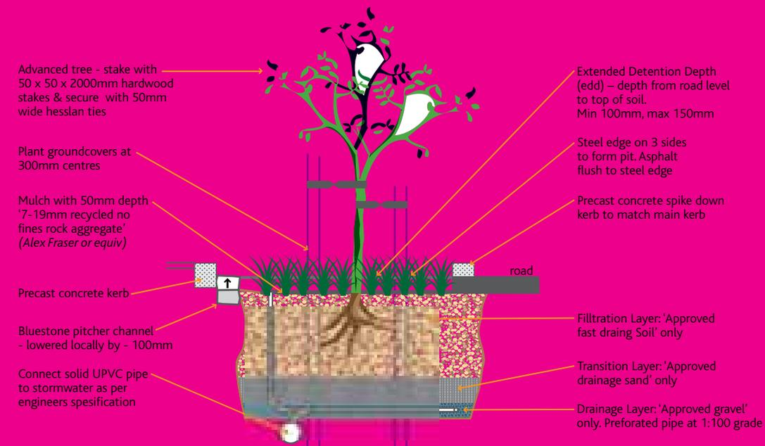
Figure 3: Plan view of raingarden showing drainage layout
