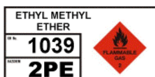
Warning notice for Dangerous Goods Bulk Store
