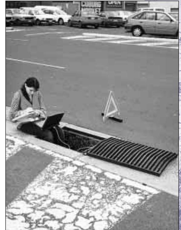
*CRC researcher retrieving data from a stormwater flow meter.*
