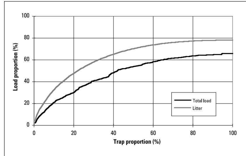
Figure 9: Plot of trapping efficiency against proportion of entrances fitted with SEPTs
