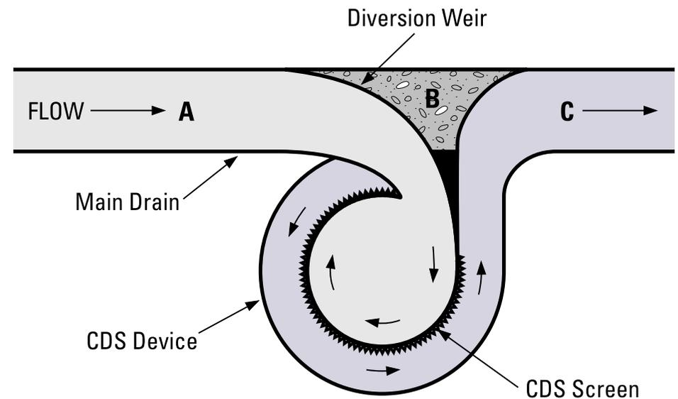
Figure 7: Diagram of CDS instrumentation layout
