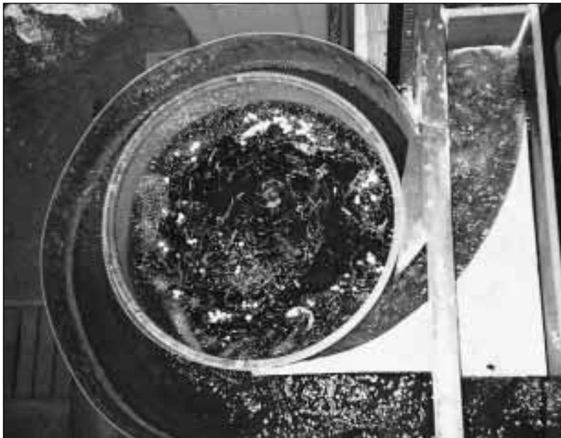
*A continuous deflective separation device (CDS) in the laboratory*
