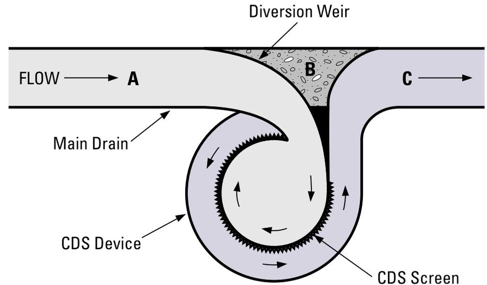
Figure 7: Diagram of CDS instrumentation layout
