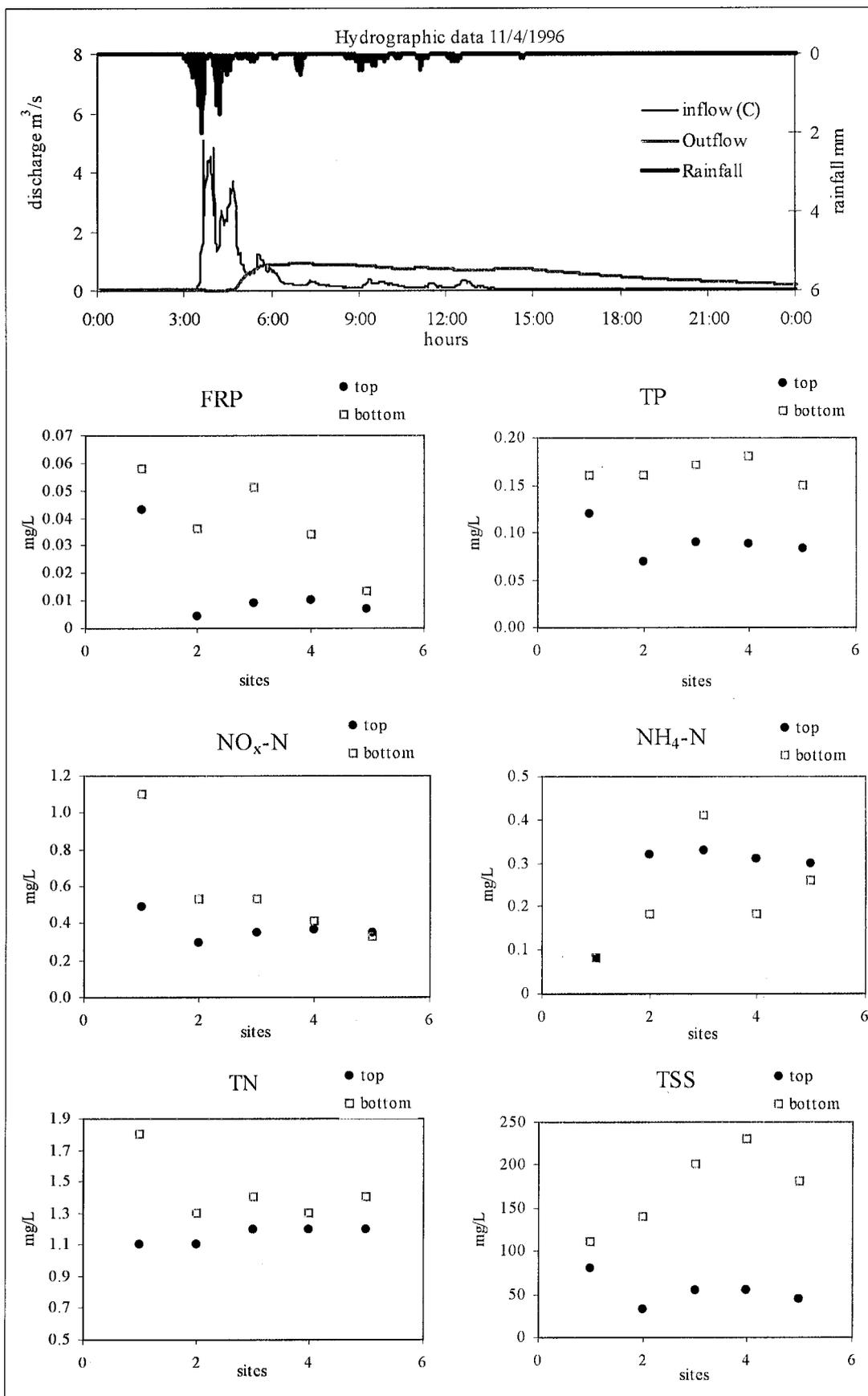
Figure 5.5 Nutrient concentrations collected during event on 11/4/1996
