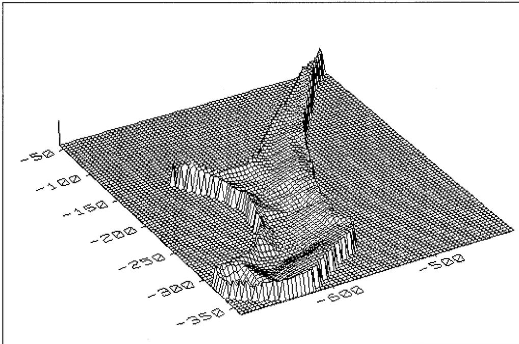
Figure 2.1 Results of Bathymetric survey of Blackburn Lake.
