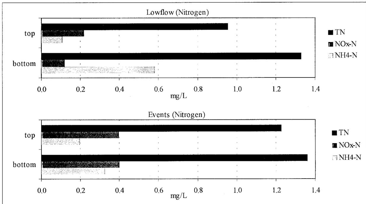
Figure 5.7 Differences between average nitrogen concentrations for low flow and event periods (sites 1-5) and differences between top and bottom concentrations.
