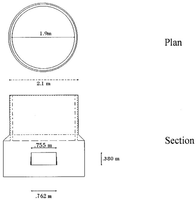
Figure 3.4 Glory hole structure at the outlet of the Lake.
