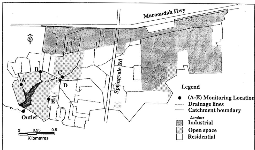
Figure 2.2 Blackburn Lake catchment boundary and monitoring site locations.
