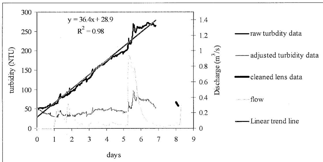
Figure 4.6 Turbidity readings affected by algae growth at the outlet. Period adjusted was 6/4/1996 – 14/4/1996
