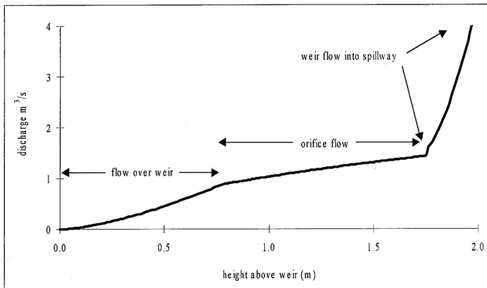
Figure 3.5 Stage discharge rating for outflow from Blackburn Lake.
