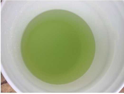
Figure 14: Light green water sample indicates high levels of algae.
