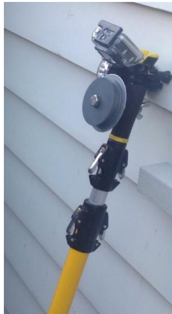
Figure 2: Mounted Camera, attached above wheel to maintain camera at 200mm above gutter while filming.
