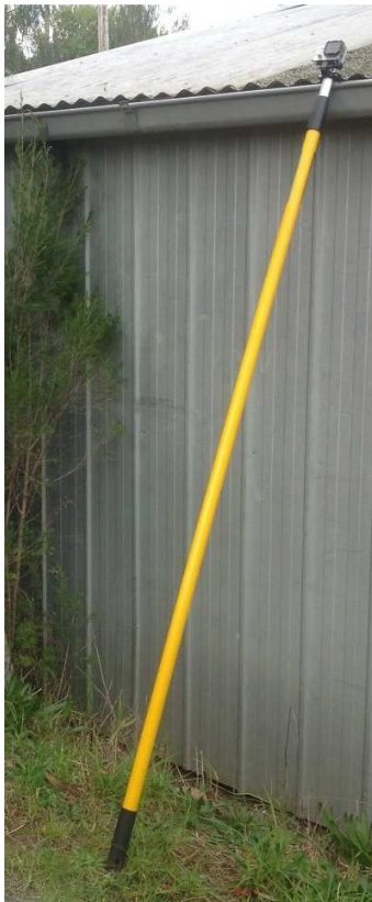
Figure 1: Mounted Camera (WiFi GoPro on a telescopic painter's pole), used to assess the condition of gutters.
