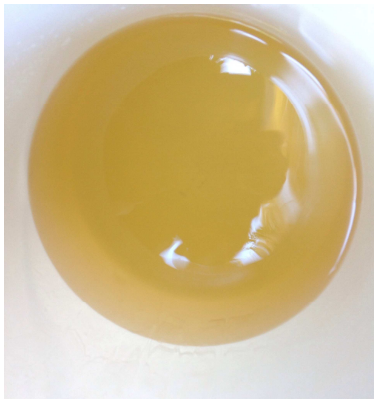
Figure 16: Light brown sample indicates high levels of tannin.
