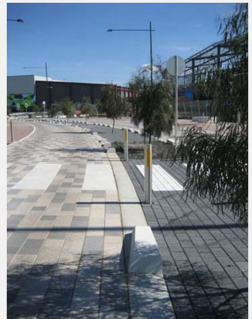
The inverted road profile allows the collection of stormwater in the centre of the road and facilitates the conveyance of larger floods (photo courtesy of Hume City Council)
