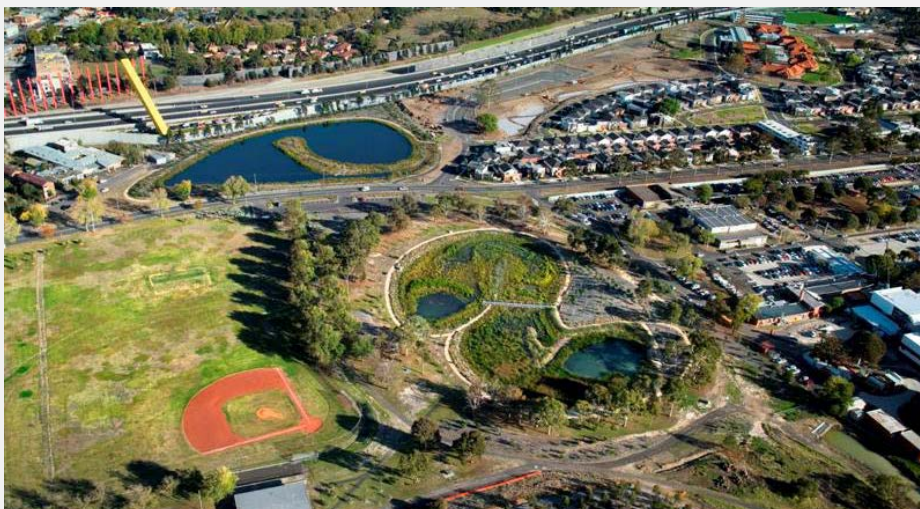
Royal Park wetland and storage basin (Photo courtesy of City of Melbourne)
